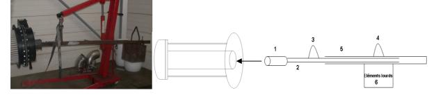
First of all, insert Part 1 into the fire tube, Mount 3 allows fitting the exchanger with a ring, then Tube 5 is moved by Mount 4 so as to adjust the system to achieve a horizontal balance. As soon as the heat exchanger is properly horizontally adjusted, it can be inserted into the hot water tank or removed without any risk of touching the sidewalls.
