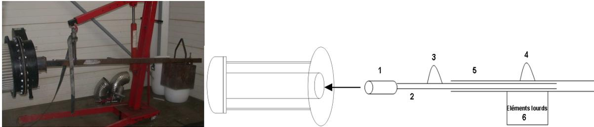
First of all, insert Part 1 into the fire tube, Mount 3 allows fitting the exchanger with a ring, then Tube 5 is moved by Mount 4 so as to adjust the system to achieve a horizontal balance. As soon as the heat exchanger is properly horizontally adjusted, it can be inserted into the hot water tank or removed without any risk of touching the sidewalls.
