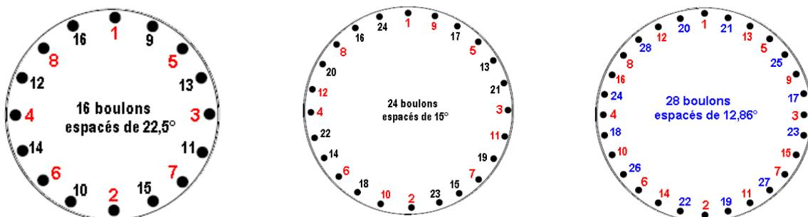
*Figures showing the tightening sequence to comply with*
