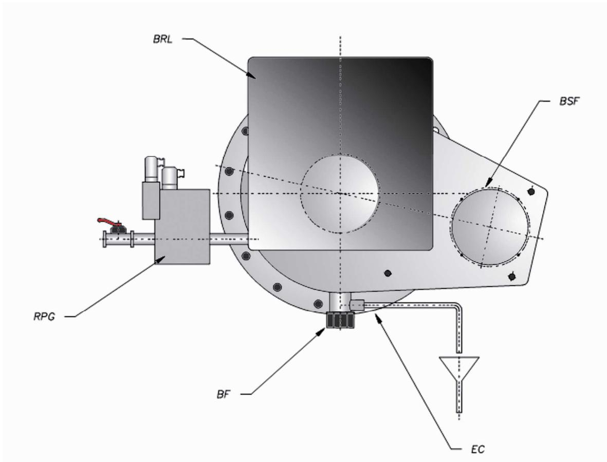
**Figure 4181.01: Condensate connection**
